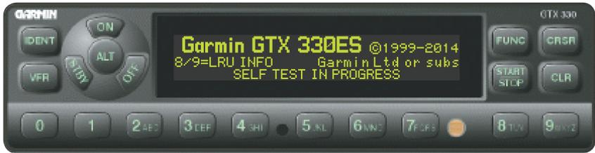
The GTX 330 transponder is powered on by pressing the **STBY**, **ALT** or **ON** keys, or by a remote avionics master switch (if applicable). After power on, a start-up page is displayed while the unit performs a self test.
