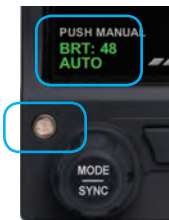
Figure 5-28 Display Brightness in BRT AUTO Mode
