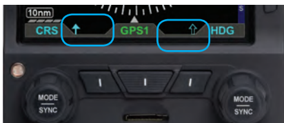
Figure 3-12 No Bearing Pointer Sources Selected
