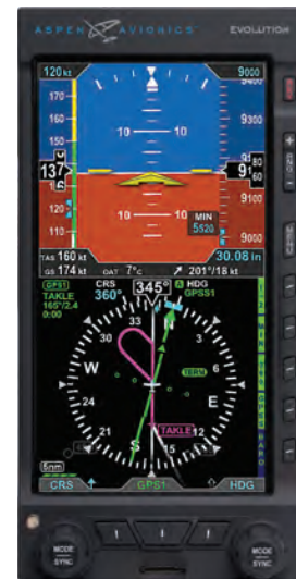
Figure 3-39 360° Mode Showing Procedure Turn, GPSS Enabled
