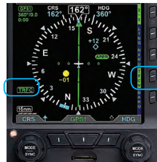
Figure 4-127 Traffic Overlay Enabled
