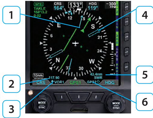
Figure 4-76 Bearing Pointer Description
