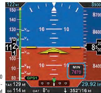
Figure 4-30 Selected MINIMUMS Field - MIN Enabled
