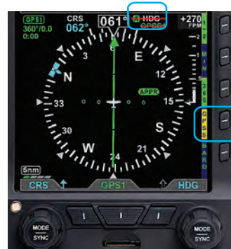
Figure 6-10 GPSS in Wings Level Mode
