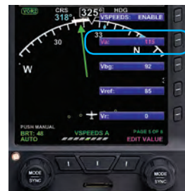
Figure 5-27 Va Vspeed Set With New Value
