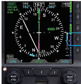
Figure 4-111 GPSS Disabled and Autopilot in HDG Mode
