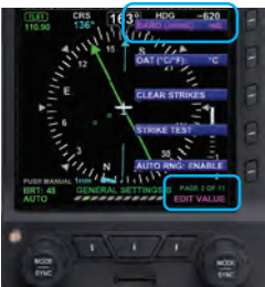
Figure 4-20 BARO Set to mB (millibars)
