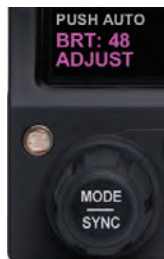
Figure 2-25 Display Brightness in BRT ADJUST Mode
