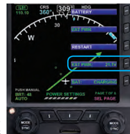
Figure 6-3 External Power Voltage Status
