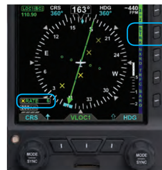
Figure 3-35 Lightning Overlay On Displaying WX-500 Strike Data
