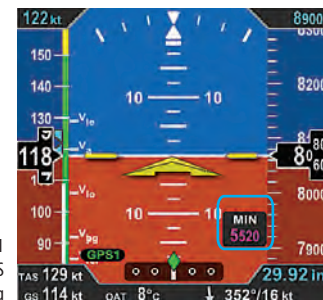
Figure 4-31 New Selected MINIMUMS Annunciation Setting
