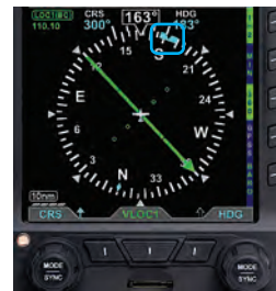
Figure 4-82 Heading Bug and Selected Heading Field
