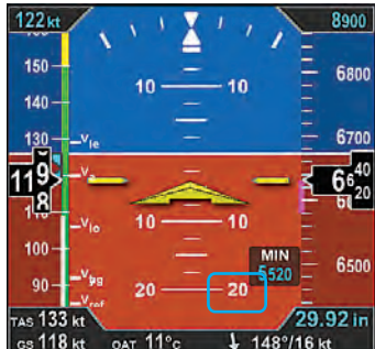
Figure 4-29 Selected MINIMUMS Annunciation and Markers Enabled
