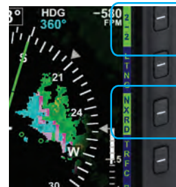
Figure 4-123 Data Link Weather Enabled
