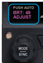
Figure 5-29 Display Brightness in BRT ADJUST Mode
