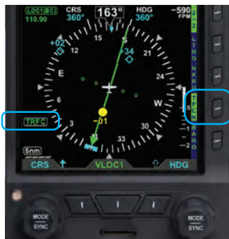
Figure 3-19 Traffic Overlay On (Traffic Normal selected)
