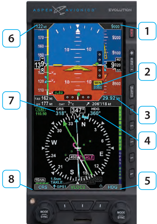
Figure 2-3 Left and Right Knobs and Corresponding Fields
