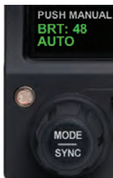
Figure 2-24 Display Brightness in BRT AUTO Mode
