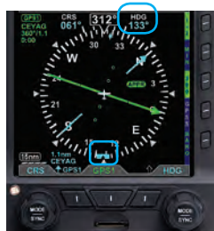
Figure 2-6 HDG field updated and inactive
