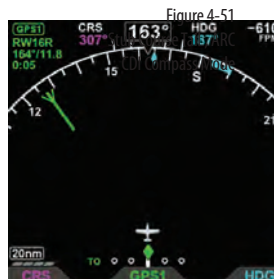
Figure 4-51 Stub Course Tail, ARC CDI Compass Mode
