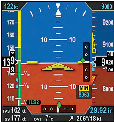
Figure 2-32 Instrument Approach Indications
