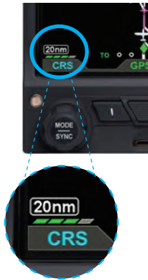
Figure 2-49 Map in ARC Compass Mode, 20nm Range at Declutter Level 3
