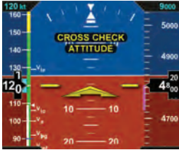
Figure 6-5 Attitude Degraded Performance
