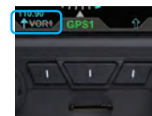
Figure 4-78 Invalid Bearing Pointer Source
