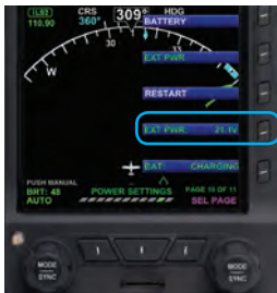
Figure 6-3 External Power Voltage Status
