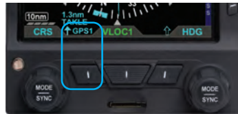
Figure 4-80 Single-Line Bearing Pointer and Button
