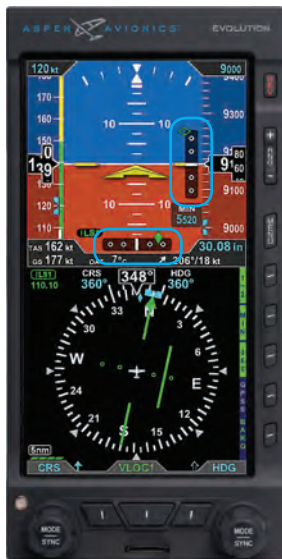
Figure 3-40 Vertical and Horizontal Deviation Indicator, Showing Glide Slope
