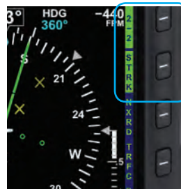
Figure 4-122 Lightning Overlay Enabled Displaying WX-500 Strike Data
