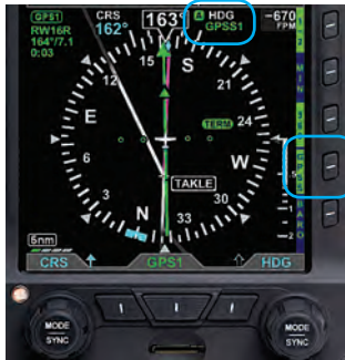
Figure 4-110 GPSS Enabled with Autopilot in HDG Mode
