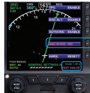
Figure 4-44 Changing the ARC Compass MODE
