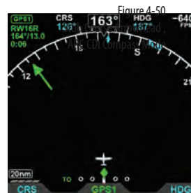
Figure 4-50 Stub Course Arrowhead, ARC CDI Compass Mode
