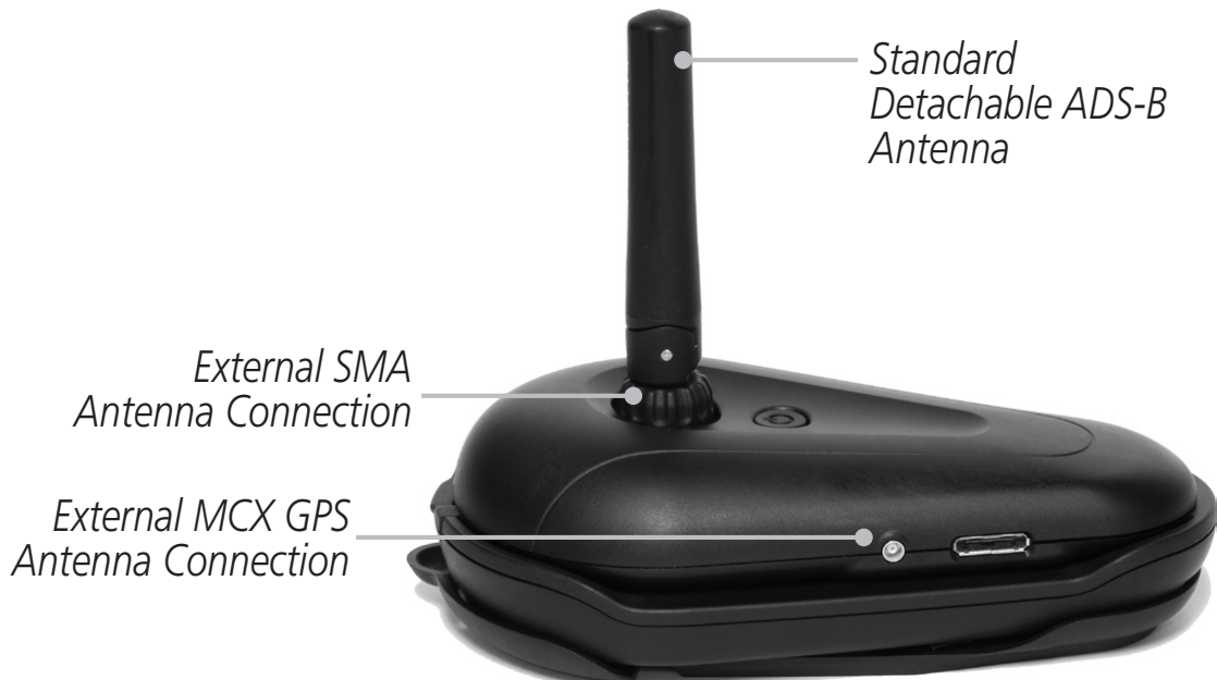
Figure 3-7 GDL 39 Antenna Connections
