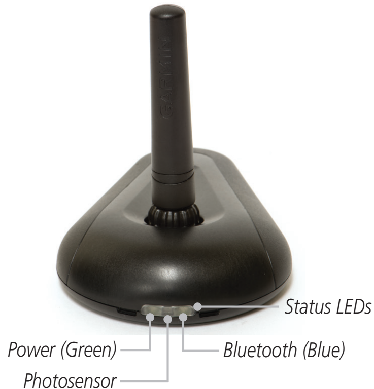
Figure 4-2 GDL 39 Status LEDs
